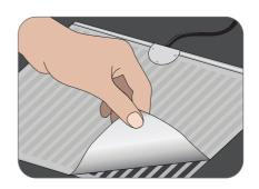
4. Position one edge of the foil on the mirror back, apply pressure evenly as the foil is gradually lowered on to mirror back.
